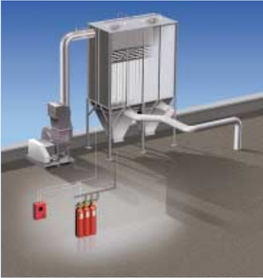
Industrial Application with SHP-PRO and CO 2 protecting a dust collector.
