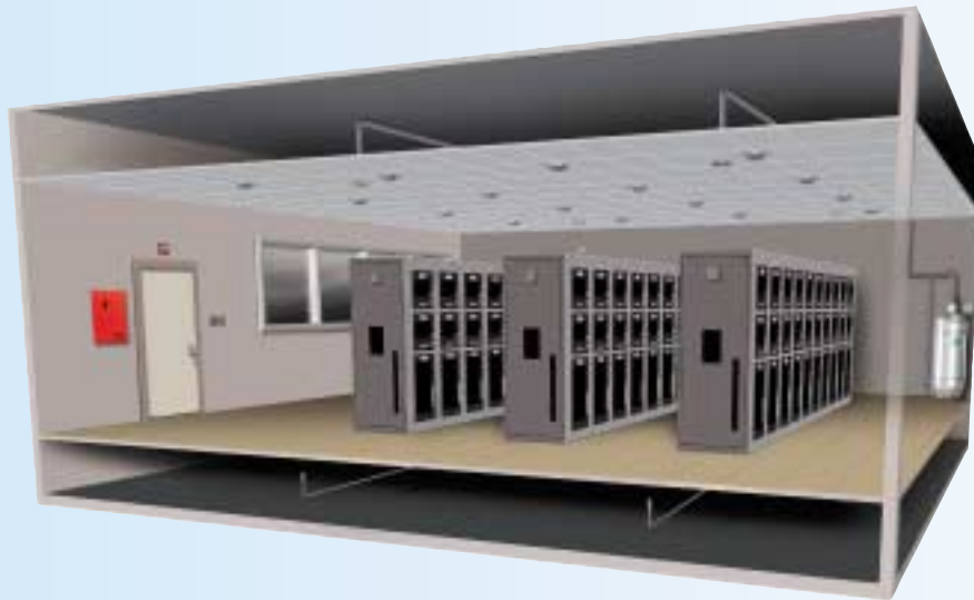
High Value Asset Application with SHP-PRO and clean agent (ECA RO-25 or HFC-227ea) protecting a Telecommunications Switch Room.
